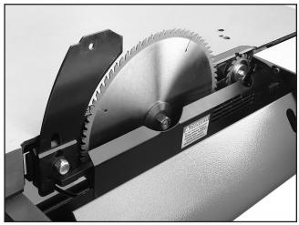
Figure 48. Internal blade guard exposed.
